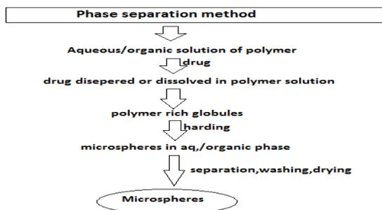
Figure 6. Phase separation method.
