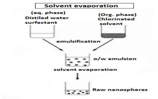
Figure 3. Solvent evaporation
