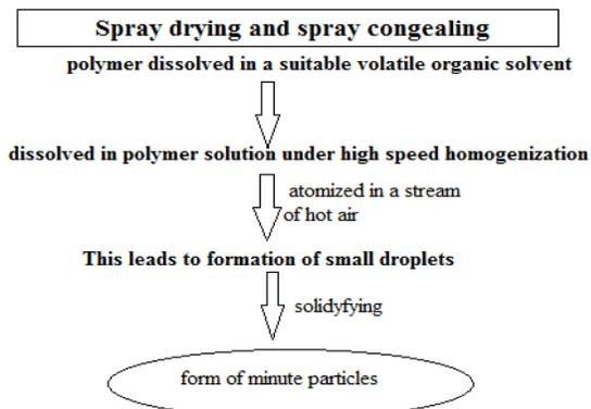
Figure 7. Spray drying and spray congealing.
