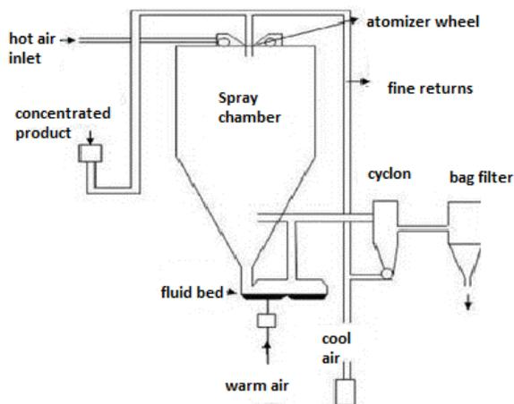
Figure 2. Spray drying technique
